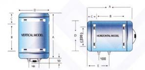
Max. Working Pressure: 0.8 MPa Rated Voltage: 220-240VAC, 1Phase
